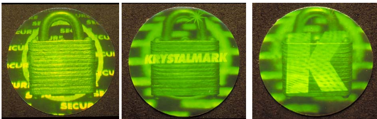
Figure 20 - Three channel volume reflection hologram at three different angles of observation. (Krystal Holographics, USA)
