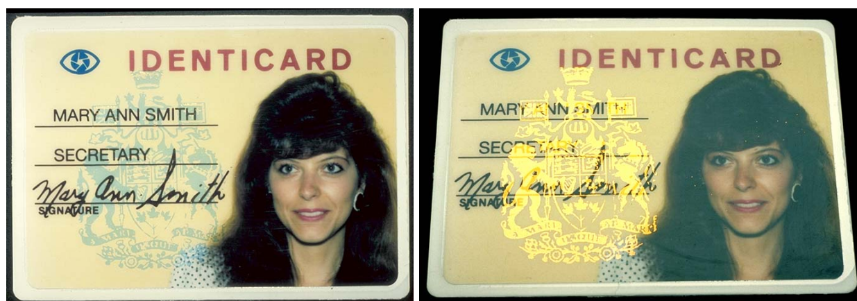
Figure 18 - All-dielectric stack at two different angles of observation: left diffuse reflection, right specular reflection. (Identocard, Canada)
