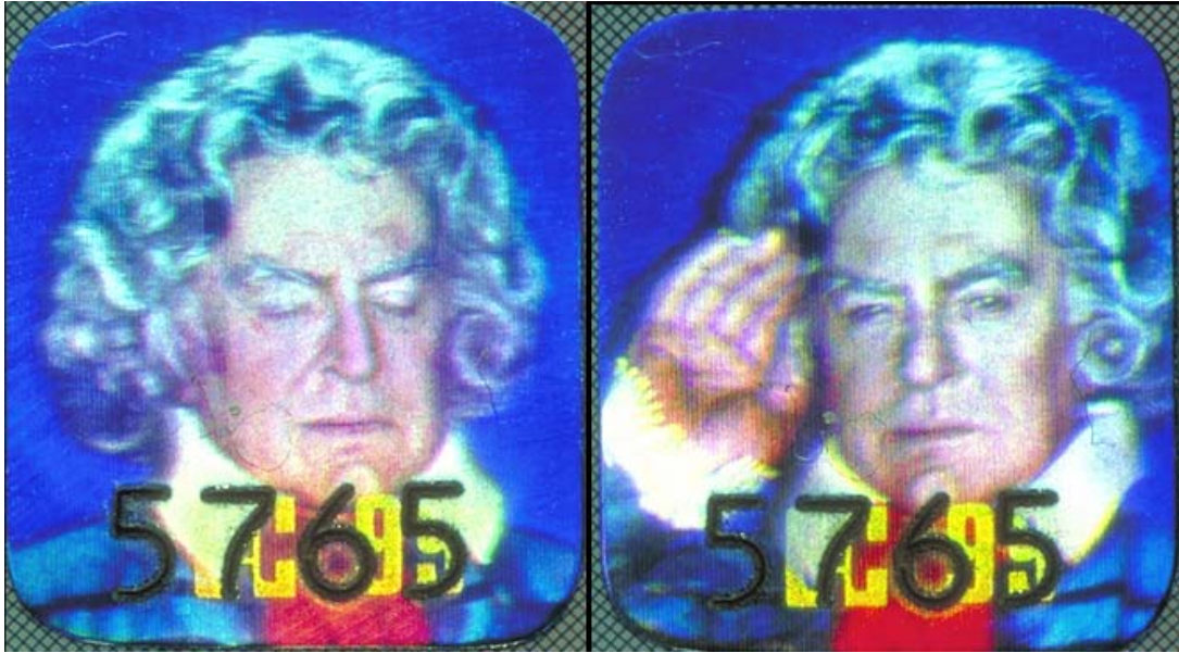
Figure 14 - Holographic stereogram: Beethoven impersonated on the hologram of the Eurocard in two different postures. (American Bank Note Holographics, USA)
