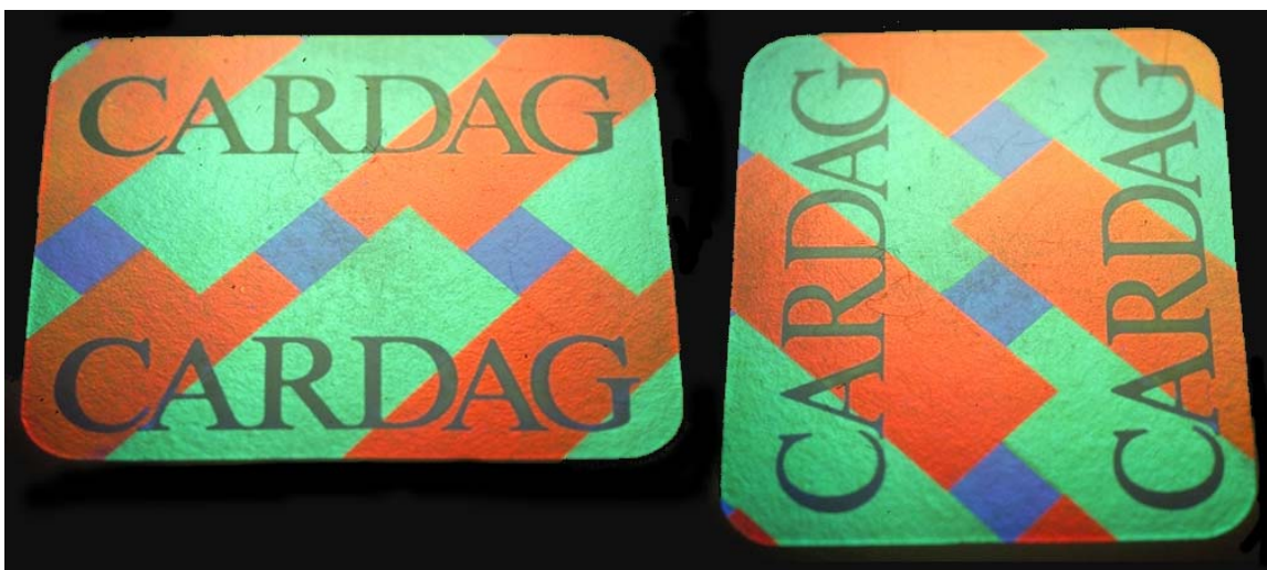
Figure 16 - The DID in reflection at two different angles of observation. Note the green to red and the red to green colour change. (Cardag, Switzerland)
