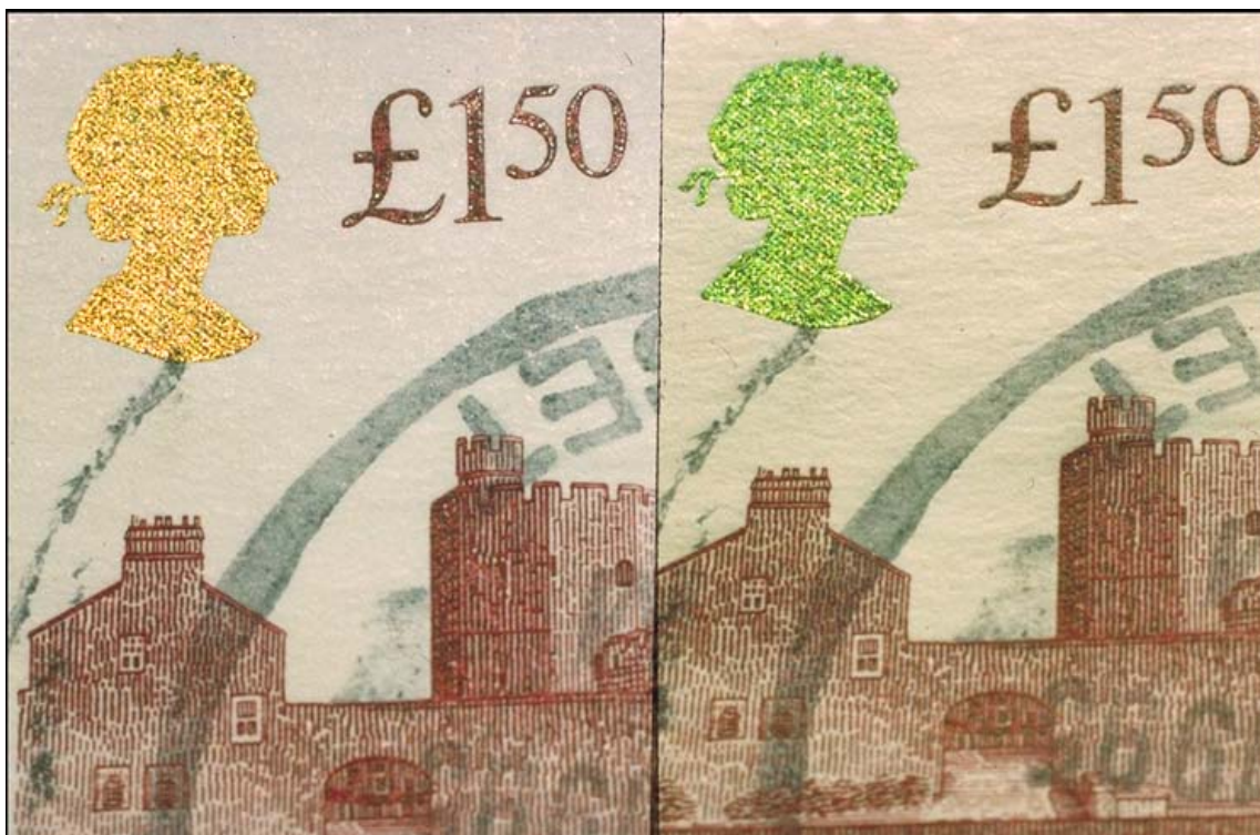
Figure 19 - Print in optically variable ink (OVI) with a gold to green shift. Left normal observation, right observation under an angle of 45^\circ with the normal. (Detail of a UK stamp). (SICPA, Switzerland)
