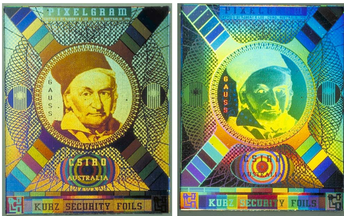
Figure 9 - A pixelgram with a continuous tone portrait: on tilting the pixelgram, positive contrast (left) and negative contrast (right) are alternately observed. (Commonwealth Scientific and Industrial Research Organization - CSIRO, Australia).
